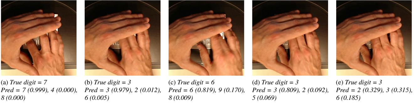
Figure 5: PIN 73633 entered by a user in our test set in the *Single PIN pad* scenario. Our algorithm suggests 73632 as the most probable PIN (probability = 21.32%), 73633 as the second most probable PIN (probability = 20.43%), and 73636 as the third most probable PIN (probability = 11.96%). The algorithm predicts the correct PIN in the second attempt.
