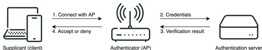
Figure 8: Components of an Enterprise network
