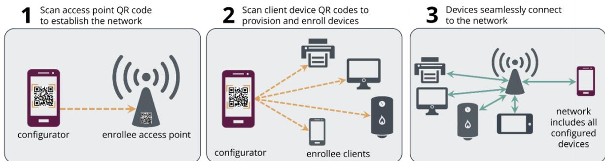
Figure 9: Wi-Fi Easy Connect - figure by the Wi-Fi Alliance
